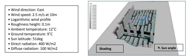
In this example, the ground surrounding the buildings, road, grass and river all have a Z depth of 2m. The ground temperature of  $9^{\circ}$ C is applied at the lower face of the ground. This represents the constant earth temperature underground.
