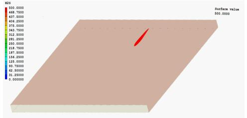
**Figure 12:** *Iso-surface of H*<sub>2</sub>*S concentration at 500 ppm*
