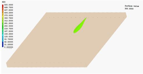
Figure 13: Iso-surface of H<sub>2</sub>S concentration at 300 ppm
