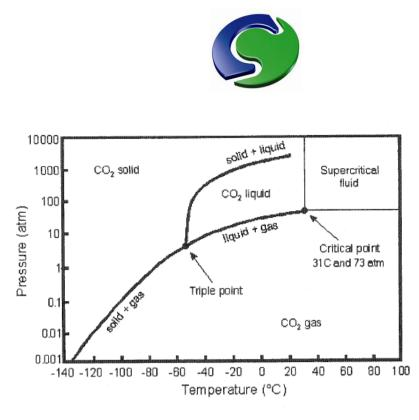
Figure 1: CO<sub>2</sub> phase diagram
