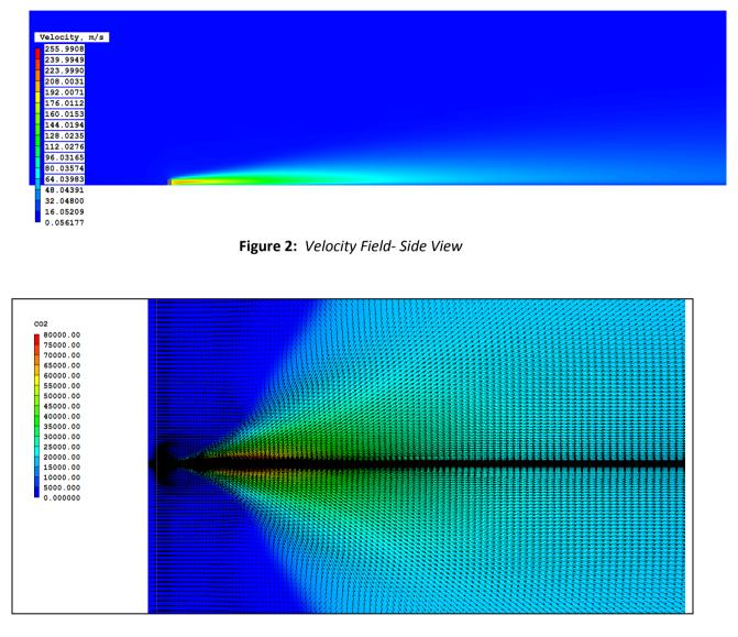
Figure 3: Velocity Field- Particular and vector field coloured by CO<sub>2</sub> ppm
