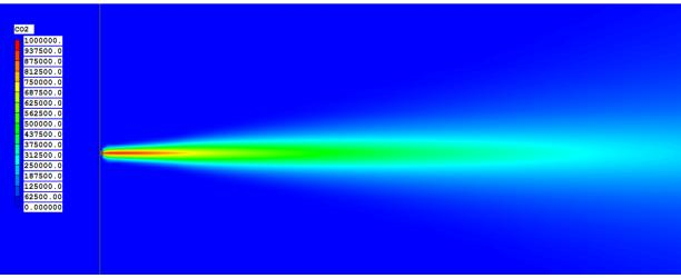
Figure 5: CO<sub>2</sub> concentration in ppm –Side view. The maximum ppm showing is set at 40000
