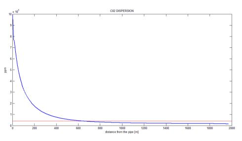
Figure 16: CO2 dispersion in the y direction. In red the 40000 ppm concentration is highlighted
