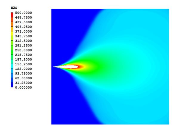
Figure 10: H<sub>2</sub>S concentration in ppm- Top view. The maximum ppm showing is set at 500ppm
