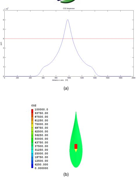
**Figure 18:** *a)* CO2 dispersion in the x direction. The red line highlights the 40000 ppm concentration. These data are taken at 470m from the pipeline indicated by the probe position in b); b)  $CO_2$  isosurface 40000ppm
