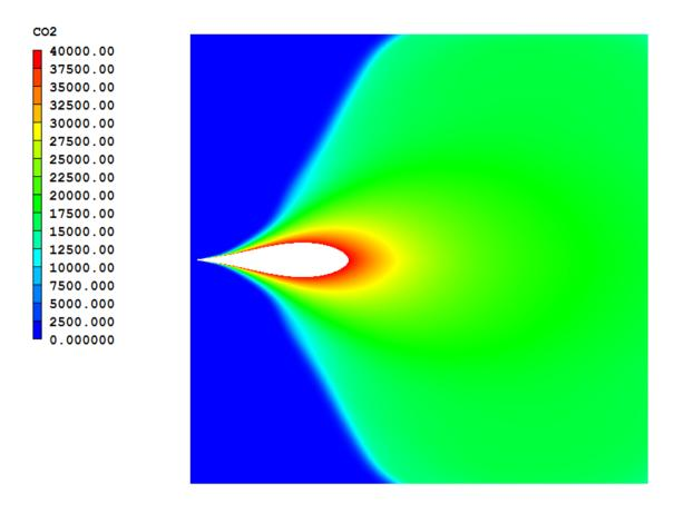
**Figure 7:**  $CO_2$  concentration in ppm – Top view. The maximum ppm showing is set at 40000
