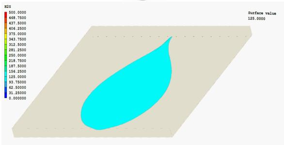
Figure 14: Iso-surface of H<sub>2</sub>S concentration at 125 ppm
