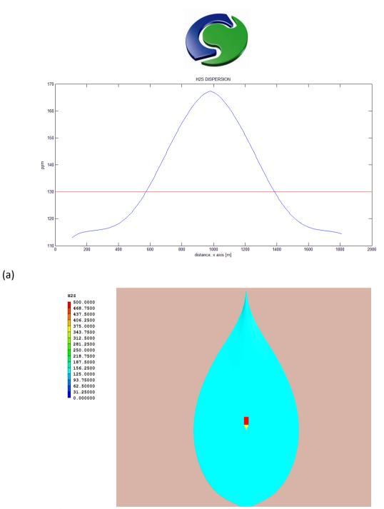
**Figure 21:** a)  $H_2S$  dispersion in the x direction. The red line highlights the 130 ppm concentration. These data are taken at 1070m from the pipeline indicated by the probe position in b); b)  $H_2S$  isosurface 130 ppm dispersion in the x direction
