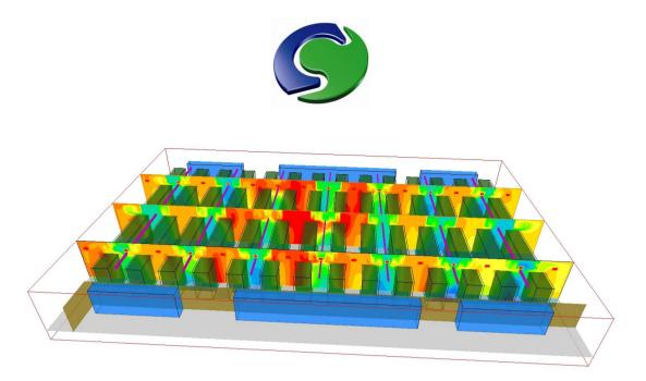
Figure 1 Temperature contours through computer cabinets (green) – under-floor and near-ceiling flow obstructions omitted
